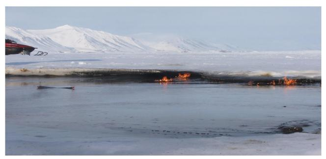
Figure 14: Burning oil on top of the fjord ice on Svalbard. Note that the burning is actually taking place under the snow/ice cover in the lateral ice cavity that was made as a result of the burning of oil. Photograph: J. Fritt-Rasmussen.
