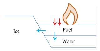
Heat loss: conduction through the sides and bottom  $\rightarrow$ Heat input: heat from flames by convection and radiation  $\rightarrow$
