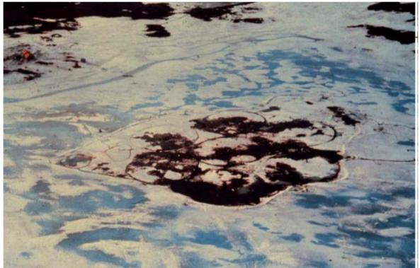
Figure 6: Oil surfacing though sea ice during the pre-melt stage during experiments of NORCOR (1975). Photo from Dickins (2011). Circles are estimated at 10-20 m diameter.
