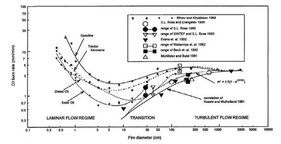
Figure 8: The regression rate of liquid pool fires (different oil types) as a function of the diameter of the pool. From Buist et al. 2013/Marine Spill Response Corporation.
