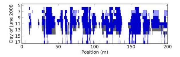
Figure 5: Development of surface characteristics along a linear transect between 5 and 17 June 2008: snow, bare ice or white, decaying ice (white); slushy ice (light blue); melt pond (dark blue); suspended ice (gray). Note the increase in meltpond coverage until 11 June (pre-melt stage), followed a decrease due to surface drainage. From Petrich et al. (2012).
