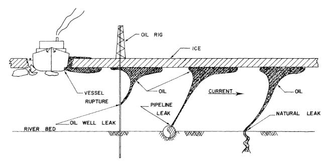
Figure 2: Schematic representation of events which could result in oil spilled beneath sea ice. From Uzuner et al. (1979).
