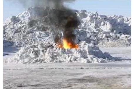
Figure 12: Burning oiled snow, that are piled into a volcano-shaped pile. From Buist et al. (2013), source Alaska Clean Seas.
