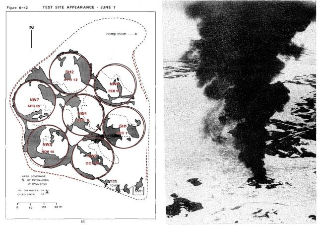
Figure 10: NORCOR test sites and oil appearance prior to burning (left) and smoke plume during burning (500 m rise) (right). Adapted from Norcor, 1975.
