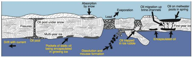
Figure 1: Sketch of oil-in-ice configurations after Al Allen (Dickins 2011).
